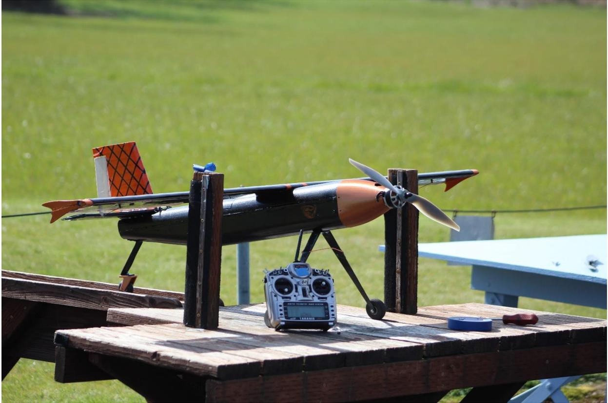
*3: Final Aircraft with full fiberglass fuselage*
