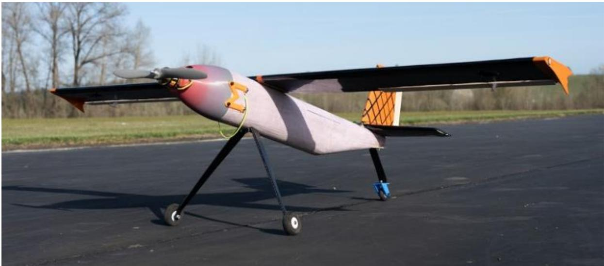
*2: Next prototype with carbon fiber wing and landing gear, and symmetrical air foil empennage*
