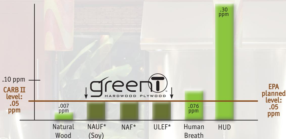
\*Each of these levels are below the CARB II requirement of .05 ppm, the most stringent emission requirement in North America.
