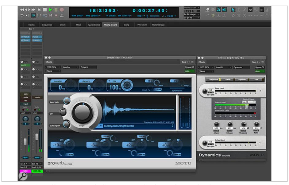
Here you see the vocal being sent through a bus to an aux track with ProVerb. Inserted on the same aux is Dynamics, with its side-chain input set to the same bus. This setup automatically 'ducks' the reverb when the singer is singing, but still leaves ambient reverb tails at the ends of the vocal lines.
