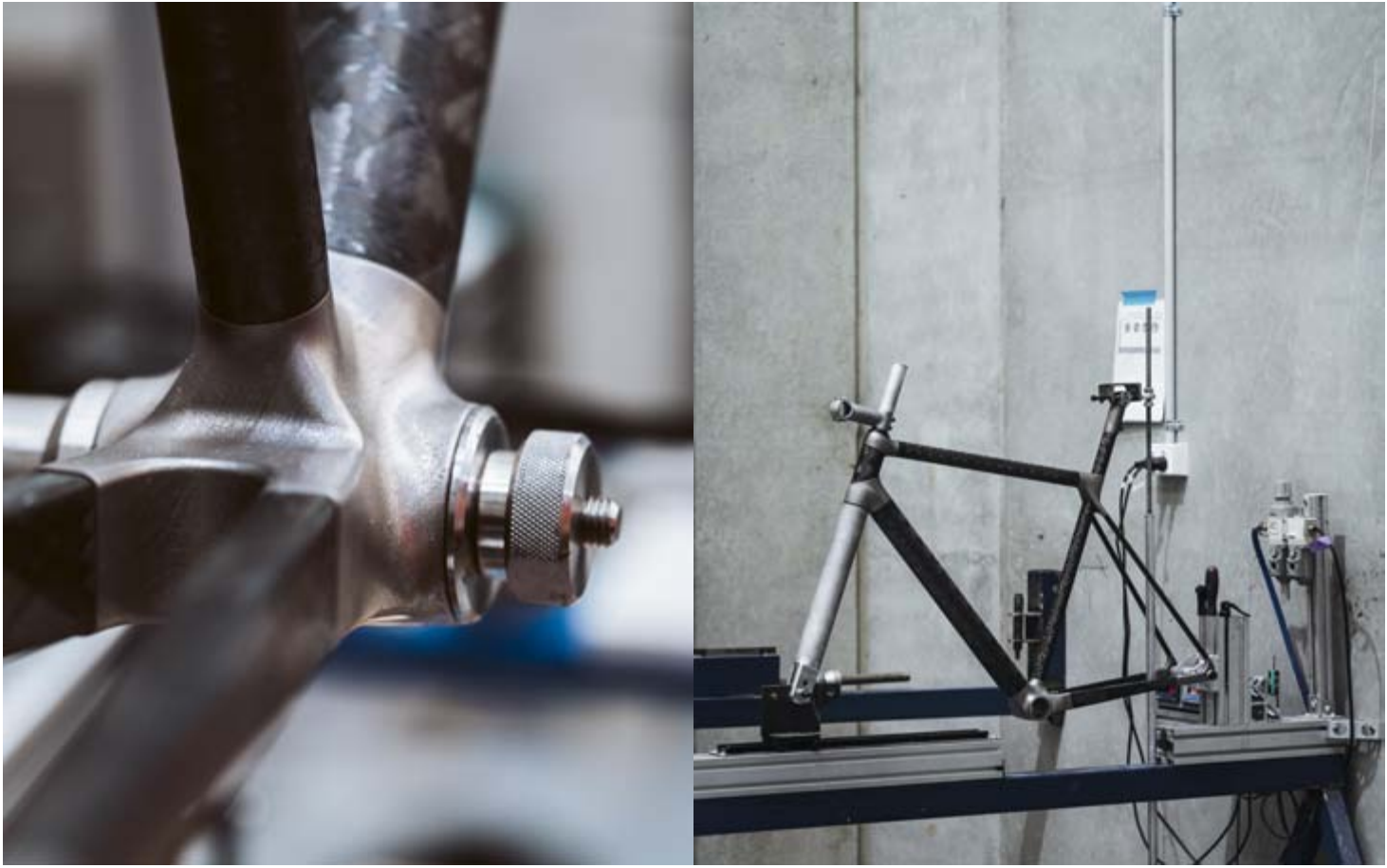
ABOVE RIGHT The lugs are 3D-printed and made up of a honeycomb structure that's 96 per cent air. ABOVE LEFT A titanium frame ensures maximum ride comfort.
