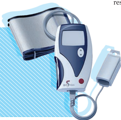
Pulsewave MAX from Biosign embeds sensors in an arm cuff and finger clip to measure five vital signs simultaneously and send that data to a cloud-based computer.
