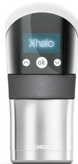
Delmedica's X-Halo compares breath temperature with core body temperature to predict when a patient is in danger of having an asthma attack.
