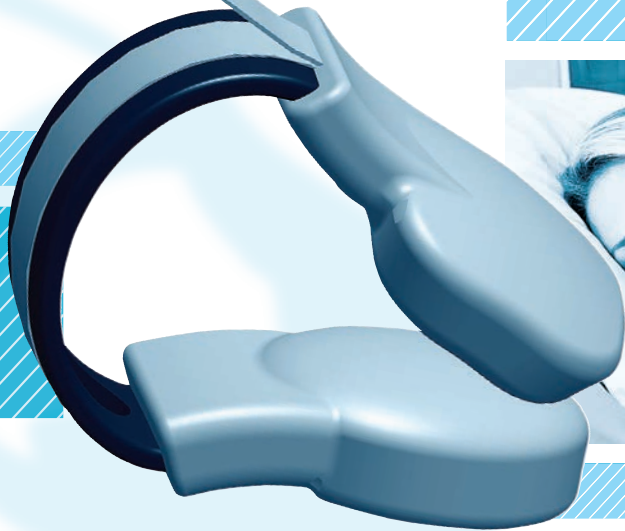
A disposable nose clip developed by Xhale measures pulse, oxygen saturation, and other cardiorespiratory vital signs. The company also makes a monitor (right) that looks for chemical markers on the breath.
