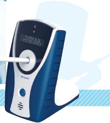
A disposable nose clip developed by Xhale measures pulse, oxygen saturation, and other cardiorespiratory vital signs. The company also makes a monitor (right) that looks for chemical markers on the breath.
