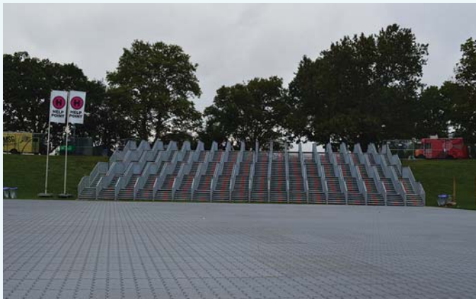
The Layher Stairway Tower 750 was specially designed to provide public access on a notable slope for last year's festival in New York.
