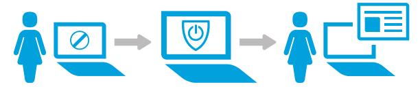
If a virus corrupts the BIOS on a notebook—preventing it from booting—HP Sure Start replaces the BIOS boot block from a separate memory within seconds, so the employee can get back to work.
