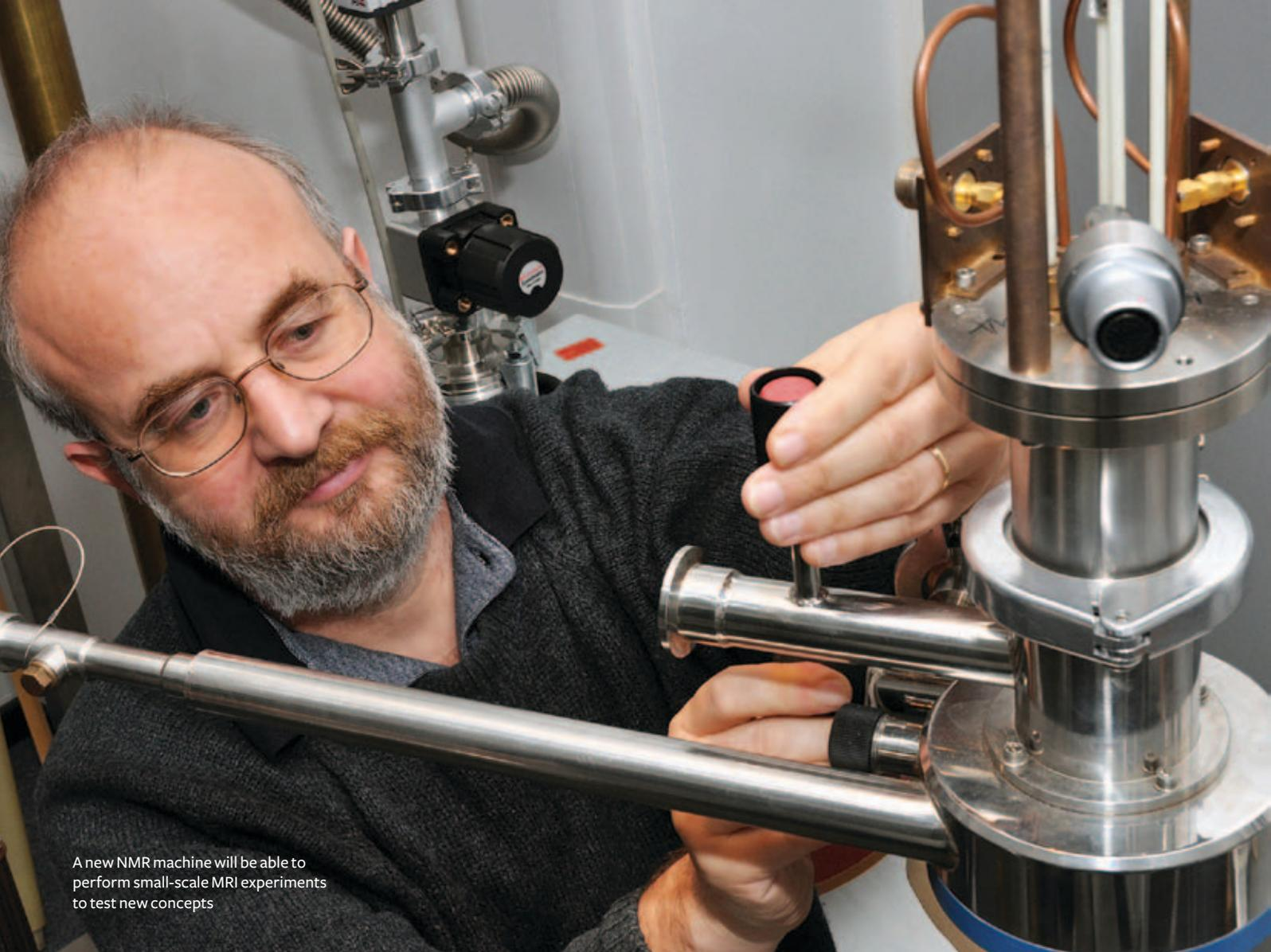
A new NMR machine will be able to perform small-scale MRI experiments to test new concepts
