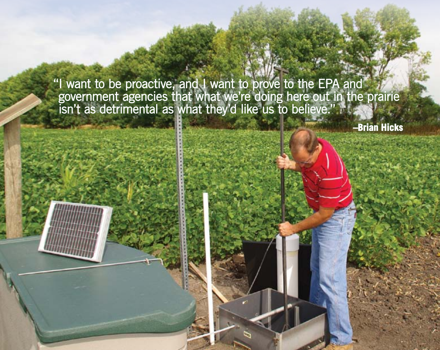
Brian Hicks tests controlled drainage on his farm near Tracy, Minn. He adjusts one of two tile outlet control structures that control the water table in this flat 100-acre field. Photo by Liz Morrison
