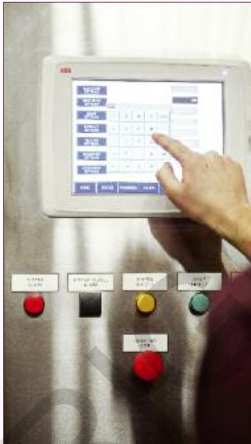
*The Tersus machine Touchscreen allows users to choose settings based on the specific qualities of the textiles being processed.*
